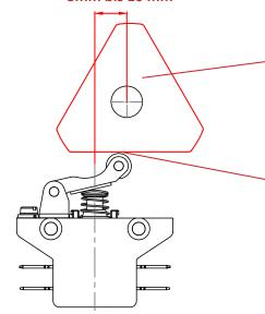
The surface of the actuator should be flat and smooth, preferably polished. The edges of the actuating edge should be round .
