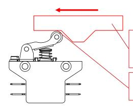
The surface of the actuator should be flat and smooth, preferably polished. The edges of the actuating edge should be round .
